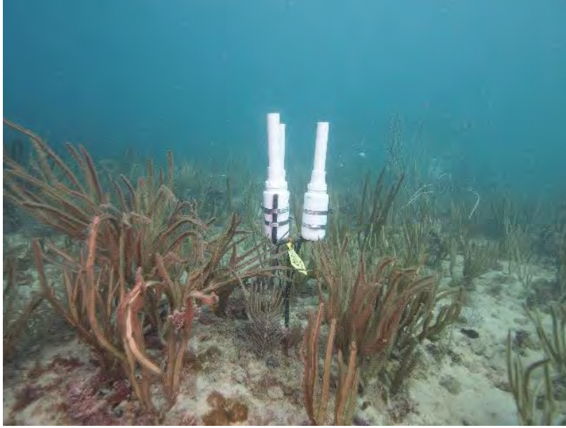
Figure 3. Sediment traps installed at all offshore sites for environmental monitoring of hardbottom and reef resources in Cuts 1 and 2.
